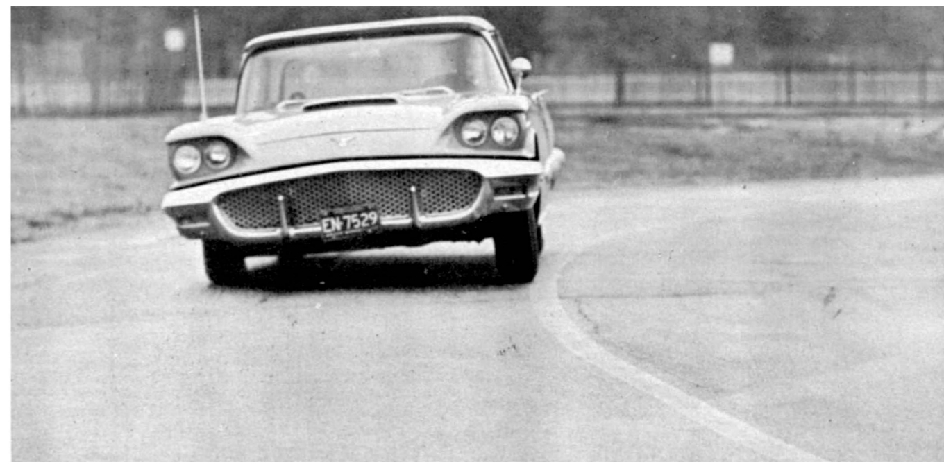
In tight bend at high speed, even the license plate leans. Inside wheel lifts; outside tire squats under heavy loading.
