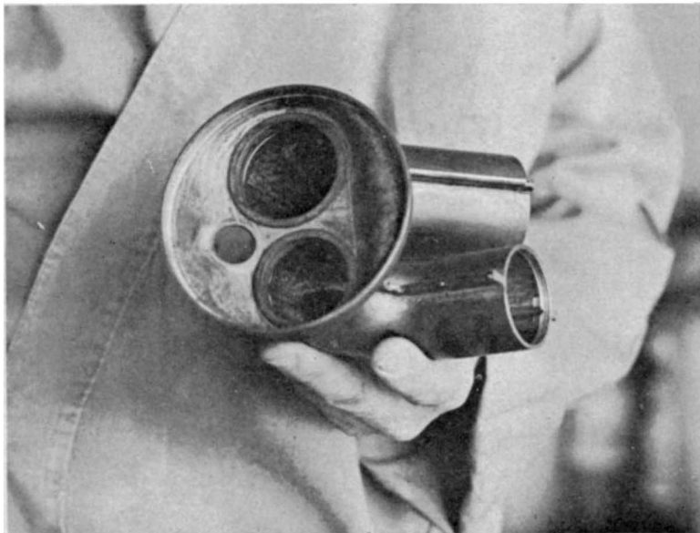
Saucer-like cylinder "head" provides wedge type combustion chamber. Fabricated ports can't miss having smooth inner surface. Spark plug insert is still to be added.
