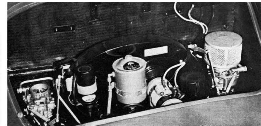
While engine lid's shape nicely suits window outline, access to forward plugs is cramped. However, engine removal is easy, even at home. New linkage, dual-throats are welcome features of new Zenith carburetors. Exhausts zig-zags to shrouded openings in bumper guards, like Detroit!
