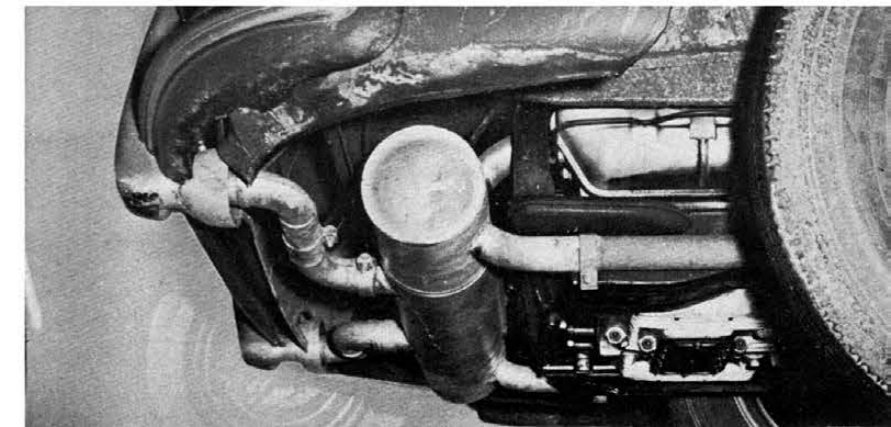
While engine lid's shape nicely suits window outline, access to forward plugs is cramped. However, engine removal is easy, even at home. New linkage, dual-throats are welcome features of new Zenith carburetors. Exhausts zig-zags to shrouded openings in bumper guards, like Detroit!
