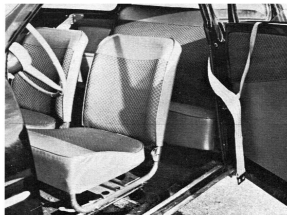
Front bucket seats give lateral support; rear seats have three-way adjustment, are "full-time" seats. Safety belts come over shoulder; released, never contact floor.
