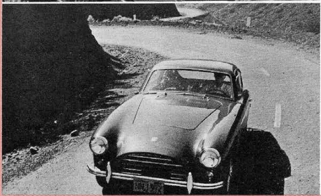
Front wheels are aligned with a slight positive camber; rear wheels with a slight negative camber, in the interests of directional straight-ahead stability. Body lines are clean.
