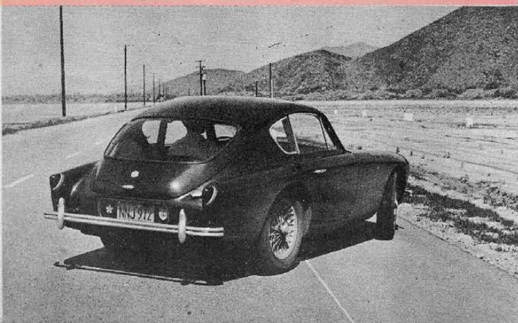
Front wheels are aligned with a slight positive camber; rear wheels with a slight negative camber, in the interests of directional straight-ahead stability. Body lines are clean.
