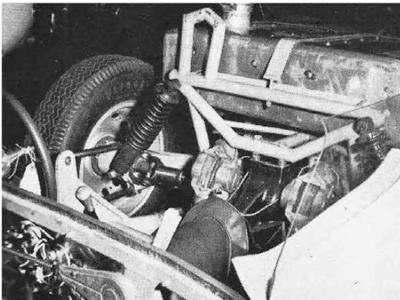
Monstrous Girling discs are clustered about the Salisbury final drive. Canted coil-shocks simplify tubular frame's superstructure.
