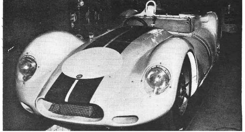
Outer slots in sleek nose blow air on front brakes; screen in center one protects oil cooler, radiator.
