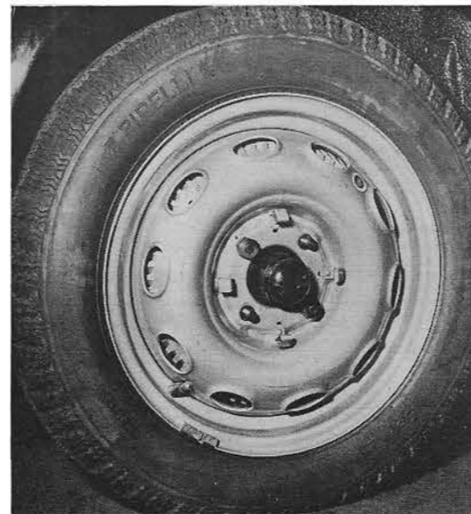
Huge diagonally-finned Alfin front drum almost completely fills inside wheel. Wheel dished, liberally vented, for air flow.
