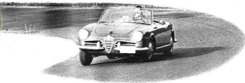
Most of the loading transfers to the outside tires, insuring lots of bite.
