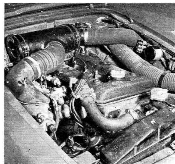
Engine is tilted a few degrees to make room for dual Webers. Collection box is fed through tubing over engine. Instrumented interior has quality tone about it.
