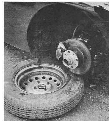
Hubs depart from past practice, using pin drive on disc wheels.
