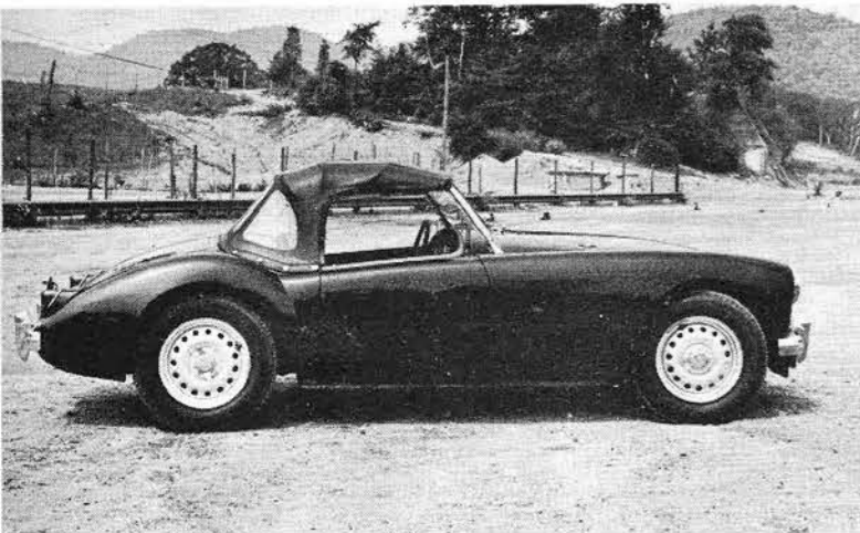
Externally the Twin Cam looks little different from the standard version except for the center-lock wheels.
