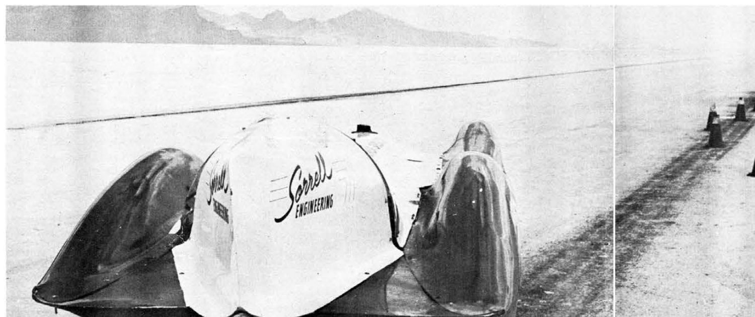
Sorrell-sponsored, Chet Herbert's 272 mph car covers its 3 injected Chevy V-8s with a Rod Schapel-shaped shell.
