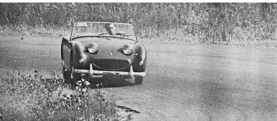
Car assumes sideways attitude as wheel is whipped into apex. The fact that car is heading at a point well inside its course indicates big slip angles.
