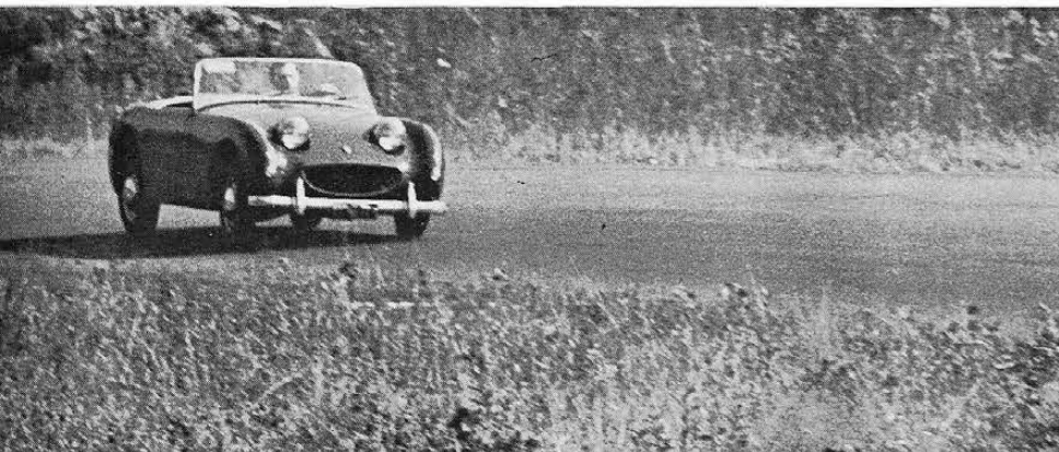
Sequence of the "new" Sprite on Lime Rock's hairpin. At approach, heavy oil in shocks keeps machine level at beginning of arc. Missing grille is our idea.
