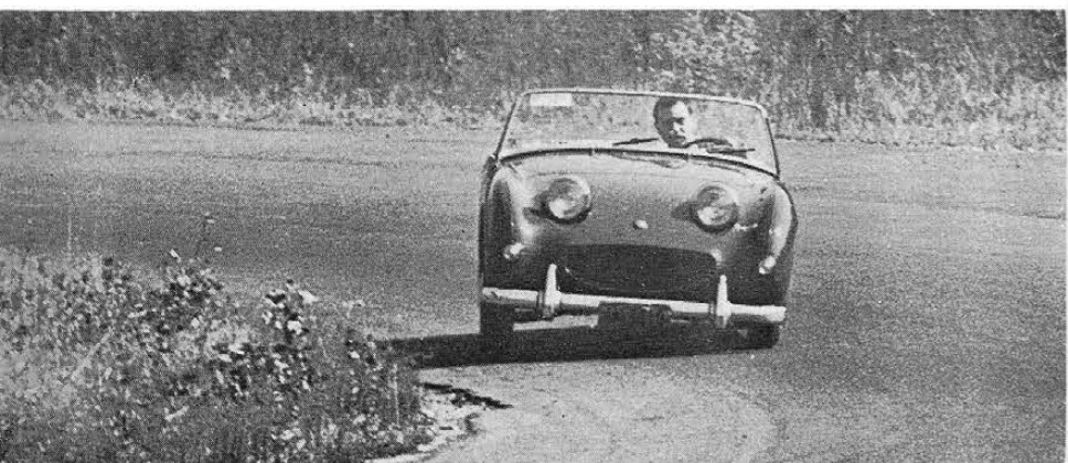
Stiffness of shocks puts car into lean gradually, and significant response to accelerator holds the drift. Under power, Sprite now surges out of corner.
