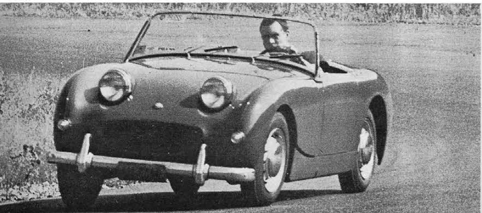
Stiffness of shocks puts car into lean gradually, and significant response to accelerator holds the drift. Under power, Sprite now surges out of corner.
