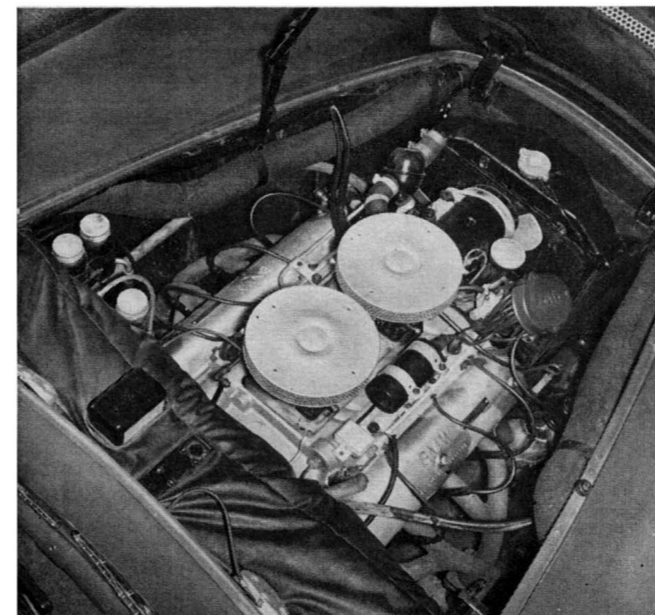
The test car's engine, the 2.5-liter BMW aluminum V-8.
