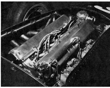
the two twin-throat Weber carburetors is attached to the right-hand cam cover and connects to the foot throttle by a series of bell-cranks and rods. The top of the radiator overflow canister can be seen at the front of the engine. In the lower photo the details of the rack and pinion steering and anti-roll bar can be seen, behind which are the Armstrong coil spring/damper units which attach to the beefed-up lower A-arm assemblies.
