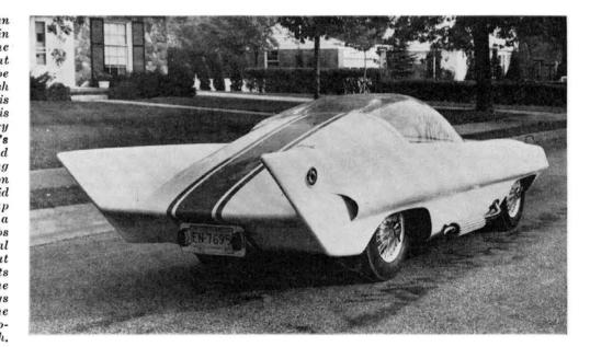
PROBLEM: to design a 1200-cubic centimeter competition sports car, with emphasis on making a dual-purpose machine embodying ease of maintenance with minimum road equipment.
