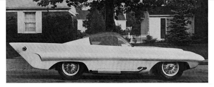
Above: the long, graceful hood and exposed exhaust pipe (a Harley Buco muffler, covered with a section of stock aluminum extrusion) are intended to express the power of the low-placed Simca "8" engine. The instrument board, simply covered with black leather, has essential gauges and no added decorative devices.
