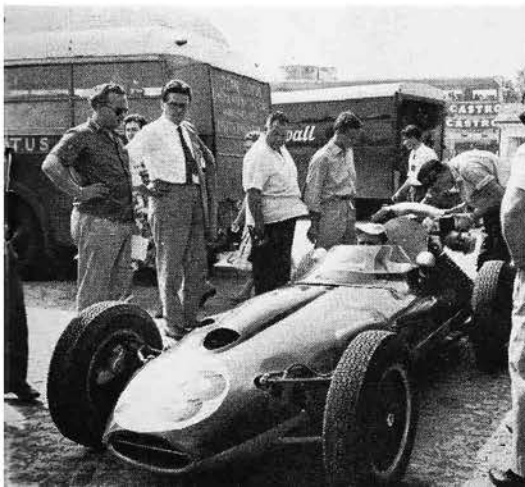
Monza Lotus had holes cut everywhere to improve cooling. Chapman (in dark glasses) looks on. Exhaust pipe was removed from original location within the body to avoid cooking driver, whose niche is snug enough anyway.
