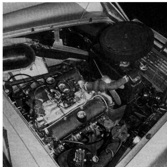
The compact, willing-to-rev V-6 asks very little room.
