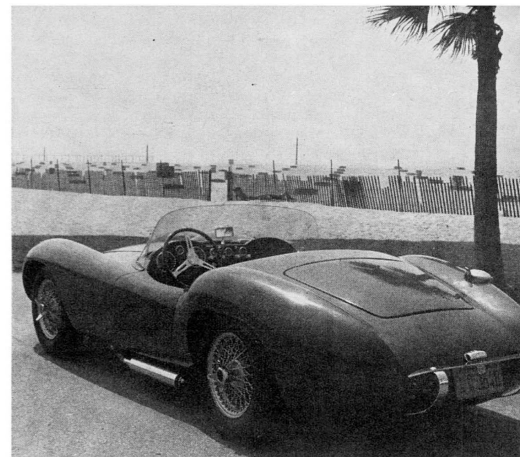
Huge gas filler cap over tank in right rear fender feeds both left and right tanks via a lower cross-over pipe between them. Total capacity is 30 gallons.
