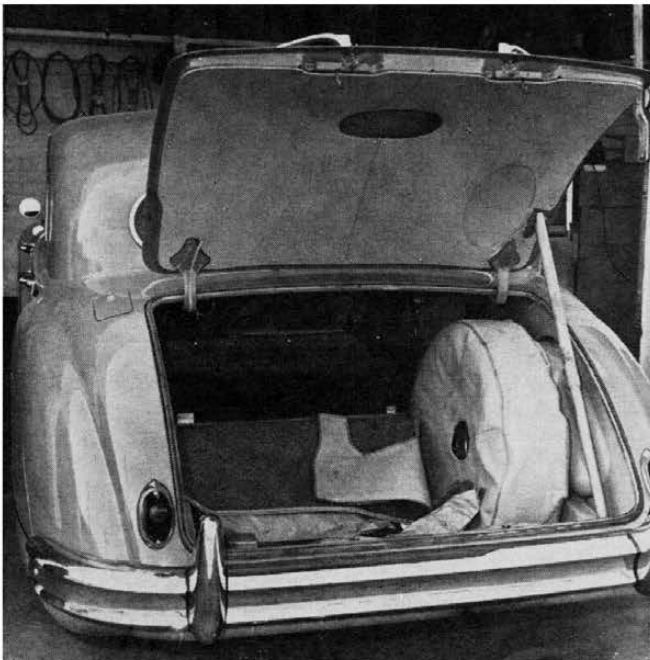
The Mark IX trunk lining is folded down to show the compact space requirement of the evaporator and blower.
