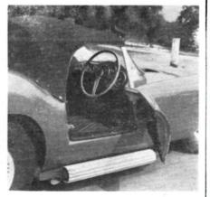
ENTRY AND EXIT are cramped. Right-hand drive is for competition, normal position is also available. Wheel is wood-rimmed.
