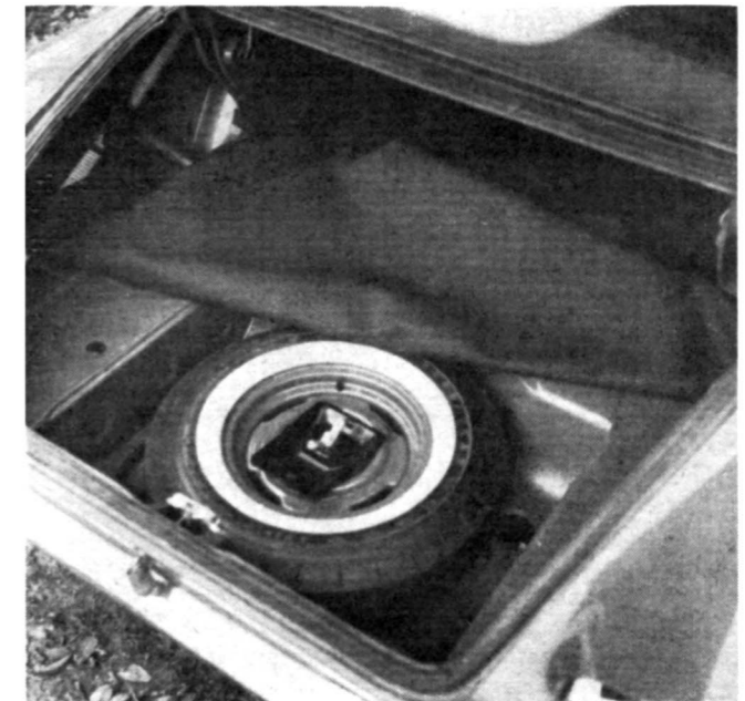
SPARE TIRE is placed underneath trunk floorboard and does not interfere with the usable luggage space. Floorboard, however, is not sturdy and will deteriorate under hard use.
