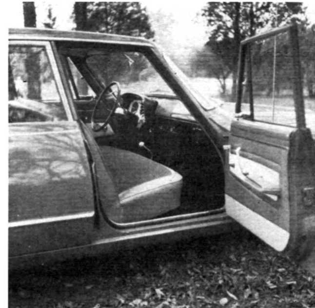
FRONT SEAT adjusts on a curved track and, when the seat is slid to the rear, tilts backward. Manual shift lever is placed in center and could interfere with third passenger's comfort.
