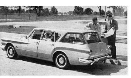
**ALL VALIANT WAGONS** are built with four doors and share unit body construction method and inclined six-cylinder powerplant with the previously announced sedan. Overall height is 53.4 inches, only one-tenth of an inch higher than sedan.
