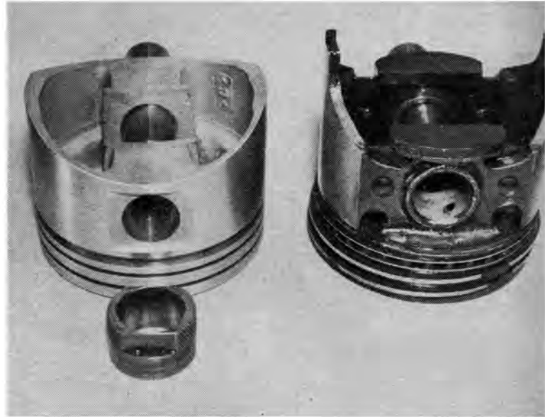
An alternative to floating the pins is one that may be used when the engine concerned is only worked on in well-equipped shops. Flats are milled onto bosses of racing piston (left) to provide seat for hydraulic press to push against using stock-type pins.
