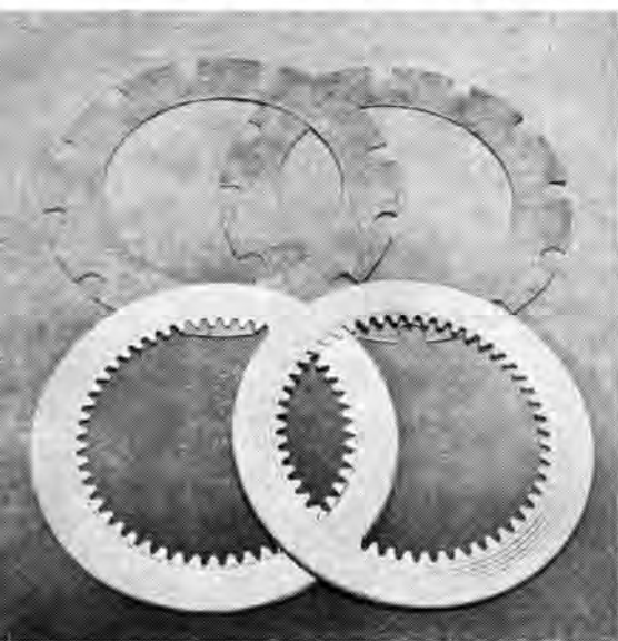
Types of driving and driven clutch plates used in Hydro-Stick box. Material on faced plates differs from standard plates.
