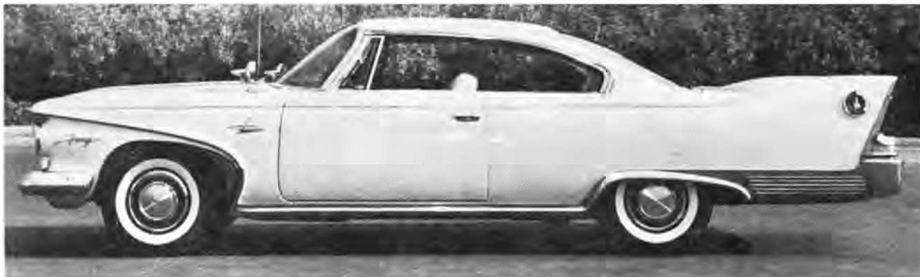
Sedan models for 1960 are 209 inches long with 118-inch wheelbase. Lowest in height is two-door hardtop model at 54.5 inches. Sport Fury test car weighed 4080 pounds but with 361-inch SonoRamic engine, needed only 7.5 seconds for 0-60 acceleration.
