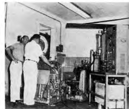
ABOVE—Extensive testing on Holman & Moody engine dyno revealed that Falcon engine is very responsive to minor changes in compression, carburetion and camshaft. Observed horsepower of stock engine was 66; with H & M Power Pack, 113 hp.
