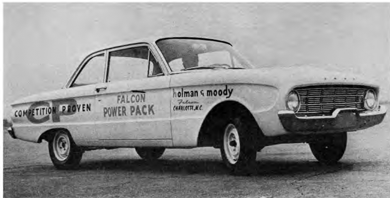
Holman & Moody-prepared Falcon with triple carburetion and cam will go from 0 to 60 mph in 13.6 seconds versus 16.1 seconds when stock. Top speed was raised from 85 to 96 mph but most important, 50-70 mph passing time dropped from 16.3 to 10.8 secs.
