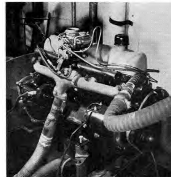
Stroppe and Associates also conducted before and after test of Falcon engine. Here, in stock condition except for larger carburetor jets and increased spark advance, the engine produced 72.3 hp at 4000 rpm.
