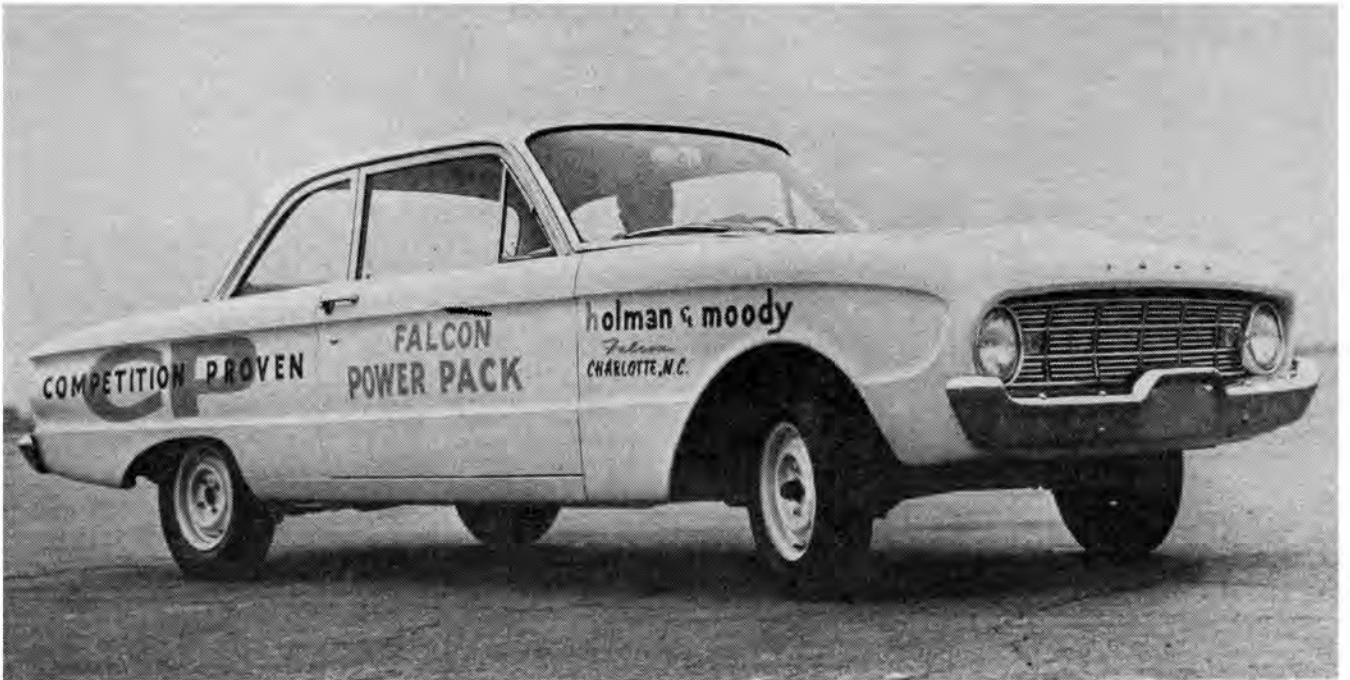
Holman & Moody-prepared Falcon with triple carburetion and cam will go from 0 to 60 mph in 13.6 seconds versus 16.1 seconds when stock. Top speed was raised from 85 to 96 mph but most important, 50-70 mph passing time dropped from 16.3 to 10.8 secs.
