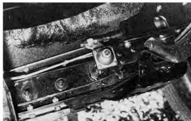
Power for hydraulic clutch actuation comes through standard Stude foot pedal linkage to '53 Chevrolet master cylinder mounted on under-bellhousing crossmember with homemade bracket. Clutch assembly is a Schiefer, uses standard Chevrolet 11-in. disc with 7/32-in. removed from front of hub for clearance.
