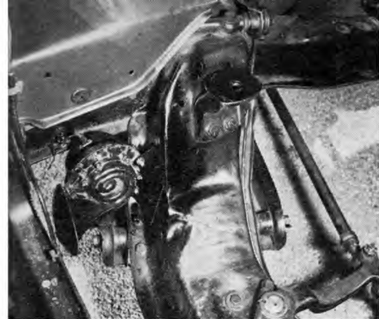
Careful placement of engine made possible using stock Studebaker frame's engine mounts after slight re-positioning. Mounting mill rather high and 1/8-inch off-center to right gave full clearance to all steering gear. Cadillac engine mount pad assemblies ('52-'56, right; '49, left) are used on '58 Chrysler block.
