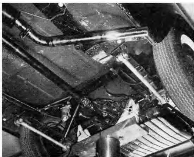
Export model Larks intended for rugged fleet use have sturdier rear ends of Packard Hawk pattern. This one incorporates limited slip differential in connection with 4.11:1 ring and pinion ratio. Traction Master radius arms team with the export model's stiffer-than-standard rear springs to curb wheel hop.
