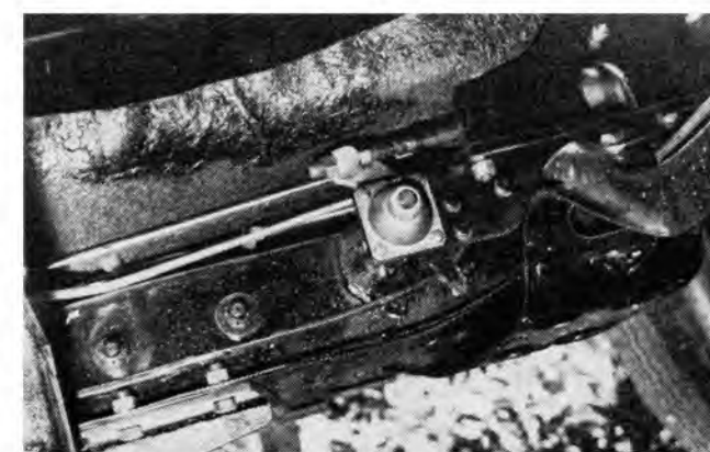
Power for hydraulic clutch actuation comes through standard Stude foot pedal linkage to '53 Chevrolet master cylinder mounted on under-bellhousing crossmember with homemade bracket. Clutch assembly is a Schiefer, uses standard Chevrolet 11-in. disc with 3/32-in. removed from front of hub for clearance.
