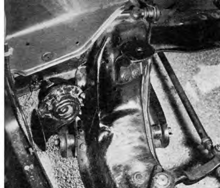
Careful placement of engine made possible using stock Studebaker frame's engine mounts after slight re-positioning. Mounting mill rather high and 1 1/8-inch off-center to right gave full clearance to all steering gear. Cadillac engine mount pad assemblies ('52-56, right; '49, left) are used on '58 Chrysler block.
