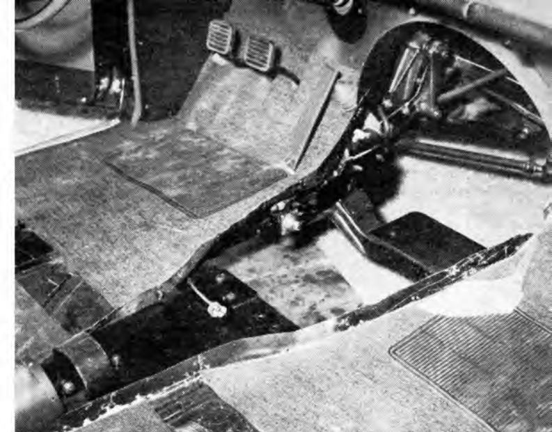
Only body alterations required were cutting larger transmission access hole, slight depression in firewall for magneto clearance. Plate bolted in center of stock crossmember is lower portion of scattershield. To its left is master cylinder for hydraulic clutch. Extension of the rear crossmember mounts driveshaft guard.
