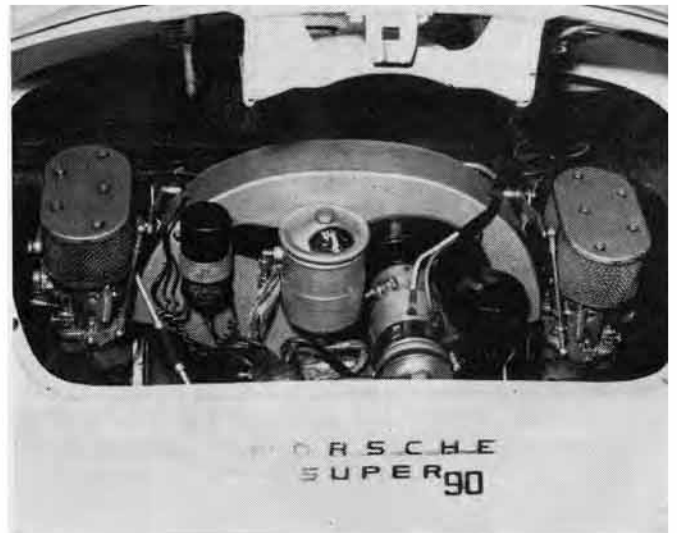
The double-throat Solex carburetors add the "super."
