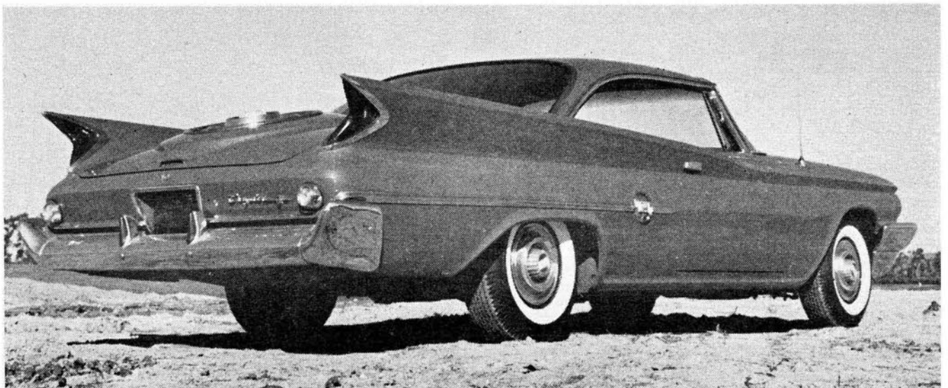
The gasoline filler neck is concealed beneath the rear license plate bracket with a 23-gallon capacity tank. 14-inch wheels are fitted with nylon Supreme grade tires. The 300F Chrysler is available for sale in only four colors; black, white, red and a burnt orange.
