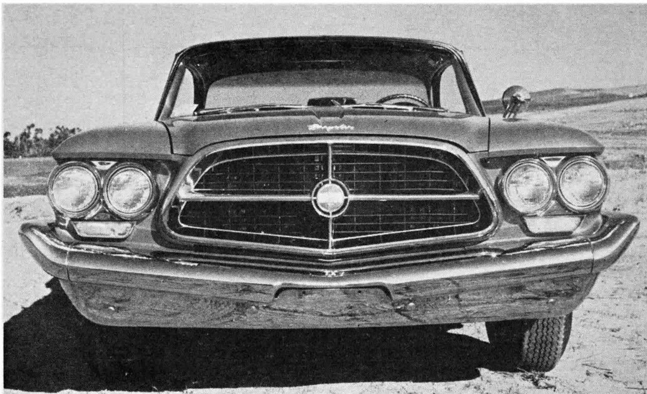
Distinctive grille opening has the 300F emblem supported by a horizontal and vertical chrome bar with a black plastic egg-crate behind. Massive front bumper wraps around the fenders for maximum protection. The hood release is operated from the dash.
