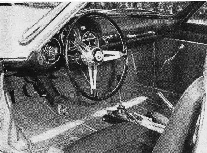
Below: The cockpit of the 850 is typically Abarth. The huge dials are well hooded, near vertical wheel allows excellent control on twisty roads. Two levers behind gearshift are for starter and choke control.
