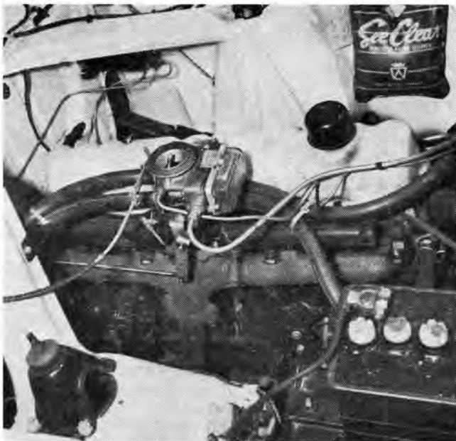
The Comet powerplant is a 144-inch in-line six with overhead valves and rocker arms. Single-throat Holley carburetor feeds fuel to intake manifold cast integrally with head. Horsepower rating is 90. Engine is an exact duplicate to one in Falcons.
