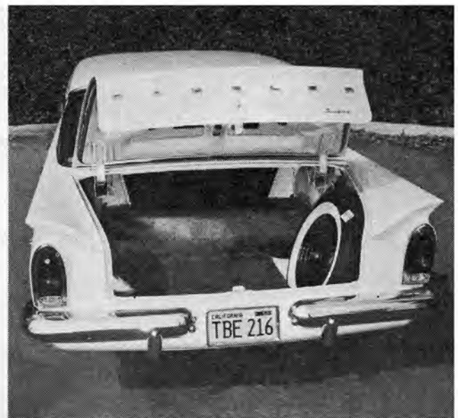
Rambler luggage compartment is spacious and has a wide opening but the curl-over portion that forms the rear panel of the car gets in the way of the head when loading and unloading pieces.
