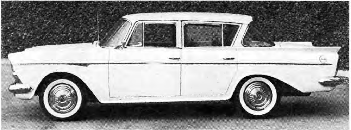
Rambler's wheelbase is 108 inches and overall length 189.5 inches. Rambler is one of the few cars made in the U.S. today still using 15-inch wheels. Larger wheels give good road clearance and excellent air circulation to cool the brake drums.
