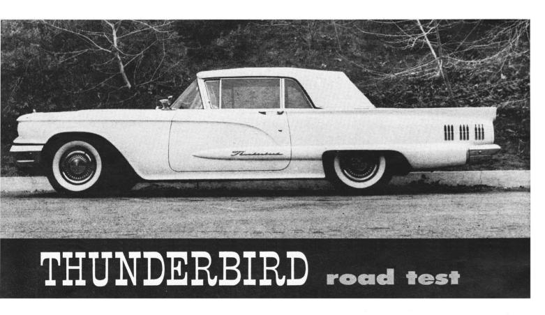
to-1. As a result, it takes careful technique to get good figures. Actual test results were o-30 in 3.7 seconds, o-45 in 6.1 and o-60 in 9.1. These do not represent the maximum capability of the 350-hp Thunderbird because this particular car was loaded down with just about every luxury option in Ford's book.
