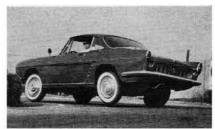
SWING AXLES of Caravelle pose problem in tight turns at high speeds. Under normal conditions, though, handling is excellent.
