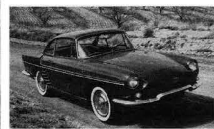
RENAULT CARAVELLE is powered by hopped up Dauphine engine, has four-speed gearbox and removable hardtop at extra cost.
