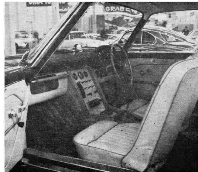
Standard instruments are in panel before driver, while others are in console between front seats. The car seats four, has plush interior of plastic and leather, and was completed in 27 days from receipt of chassis.
