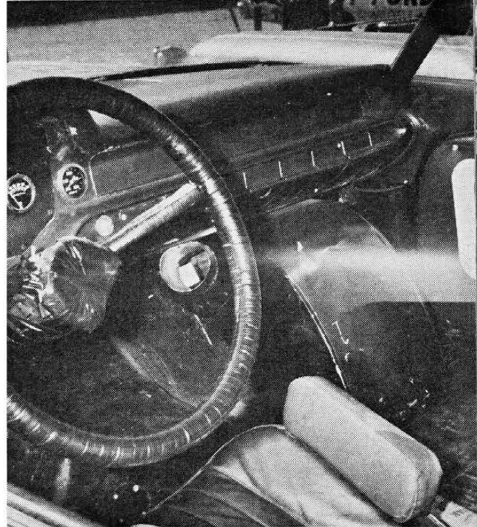
The large sheet metal bulge (where the passenger's feet would go) is one of two ducts (see photo, lower left) to cancel out negative pressures created at speed in the engine compartment. The small tube to the outside is so the driver can see the condition of the right front tire.
