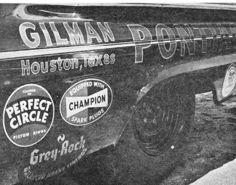
Wheels are standard-locking, but are wide-rim and use a double center for reinforcement. Tires are special racing 8.00 x 15s, using varied pressures depending on their location: at front—45 left, 65 right; at rear—55 and 60. The extra-long shocks have to protrude somewhere and so they do—into the trunk—with the bottom half of
