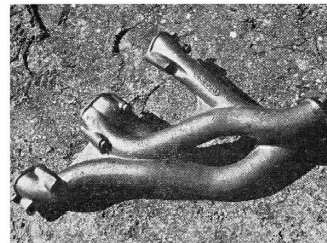
Exhaust headers used on the hot Pontiacs are huge cast-iron "tuned" headers specifically manufactured for use on racing stock cars. They are designed to scavenge the exhaust with no back pressure, the left bank header (seen
