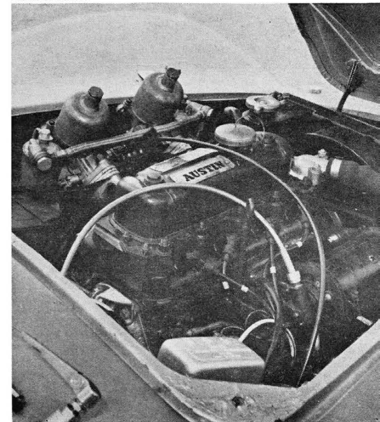
Engine is tuned to Sebring specs, using flat-topped 9.25 to 1 pistons. Tuned exhaust replaces stock manifold; 1 1/4-inch SU carbs have special intake system.
