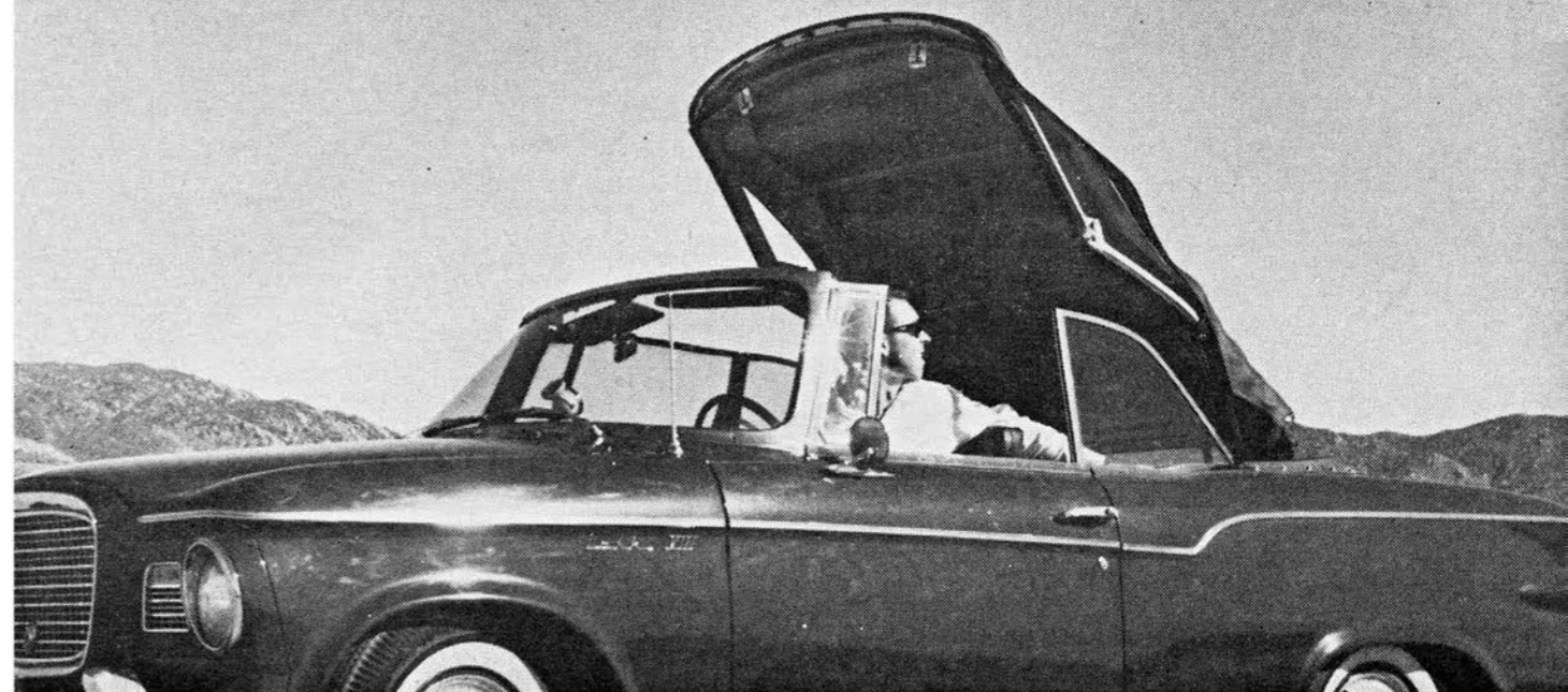
Power-operated top, standard equipment on all Lark convertibles, folds neatly into compartment behind rear seat. Two rugged latches on upper windshield frame clamp the leading edge of top against grooved rubber sealing strip.
