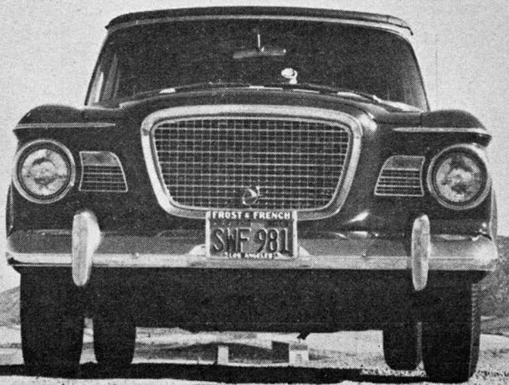
Head-on, the Lark VIII convertible resembles other hardtop models. Only major front-end styling change for 1960 is new chrome texture for grille and vents.
