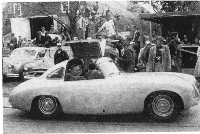
First 300SL prototype (above) had a much simpler shape than later cars. Wind tunnel testing of this form showed the need for side vents to relieve under-hood pressures. These were included in production versions. New Roadster body (below) has conventional doors and fair-sized trunk.
