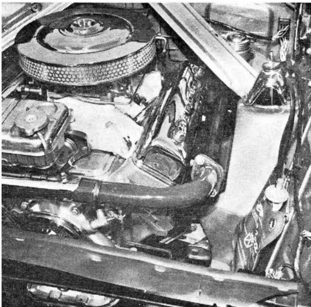
Stock exhaust manifolds and crossover pipe between the manifolds were porcelainized to help muffle noise, a single exhaust pipe used. Reworked fender wells have ample clearance around manifolds but special wrench is needed for some spark plugs.
