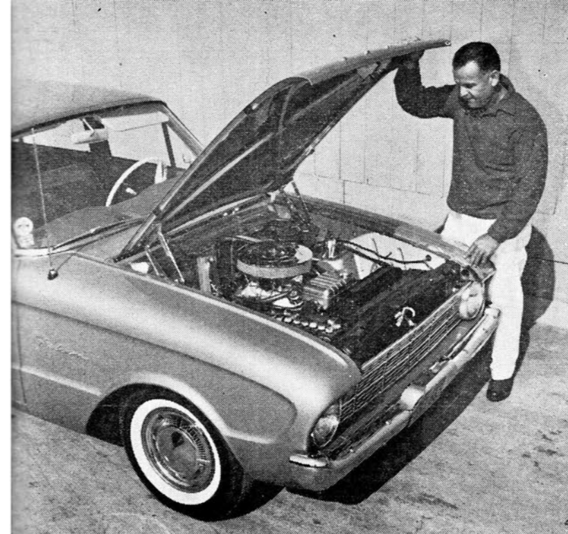
Bill Stroppe makes the final inspection of the Falcon before turning over the keys to William Ford, Vice President of the Ford Motor Company. The Merc engine occupies the same relative position in the chassis as the Falcon six. No modifications were required for hood to clear V8, accessories.
