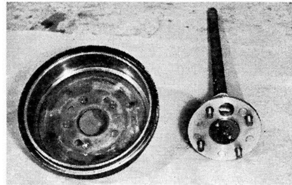
A complete '59 Ford rear axle assembly bolts directly to the Falcon rear springs with only a one-inch increase to rear wheel tread. Shock absorbers are Monroe. Ford axles and brake drums were modified (below) to match Falcon 4-bolt pattern.
