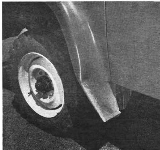
BENT FRONT FENDER resulted from creeping over rocks in order to clear front differential. Fender is actually lowest clearance.
