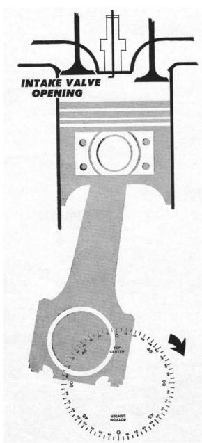
travel on the exhaust stroke. This illustration demonstrates the crankshaft, connecting rod and piston relationship at the 40 degree early opening used in some racing engines. Modern economy engines, however, may not open the intake valve until the crank rotation is some 15 degrees before top dead center.
