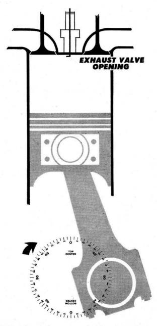
MANY RACING engines start opening the exhaust valve at 80 degrees before the end of the power stroke. The expanding gases have done most of their useful work at this point so they must escape to prevent inhibiting the pistons' upward travel on the exhaust stroke. Economy engines, designed for low rpm efficiency, don't open valve until 45 degrees before end of stroke.
