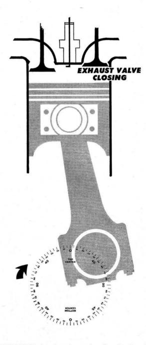
MODERN ENGINES close the exhaust valve after the piston has started down on intake stroke. This late closing can range between seven and 40 degrees depending on whether racing or economy timing is employed. The 40-degree late closing of the illustration coupled with a 40-degree early opening of an intake valve produce 80 degrees of overlap, poor idling characteristics.
