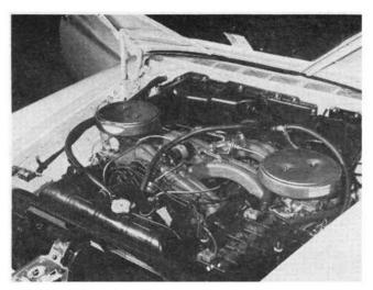
**RAM INDUCTION** is the big power plus that has added horses and torque to the 1960 Chrysler picture. Such innovations have kept both Chrysler and De Soto well in the not-so-dead power race.
