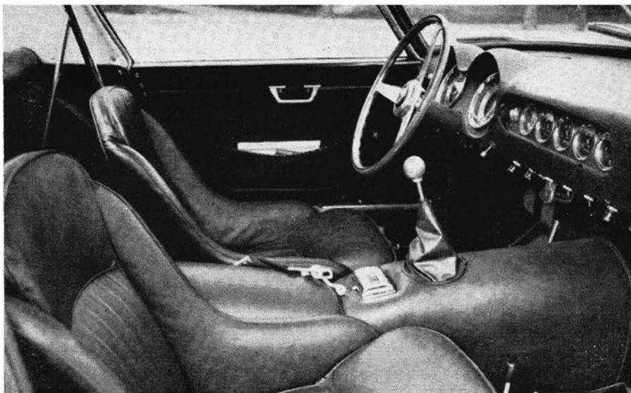
Comfortable seating for both driver and passenger plus well-finished interior mark the Berlinetta as a true dual-purpose car. It is one of the few machines that can win major races in "production" tune. Hand-filling knob on gear lever is close to wheel rim, which is arm's reach from seat back.
