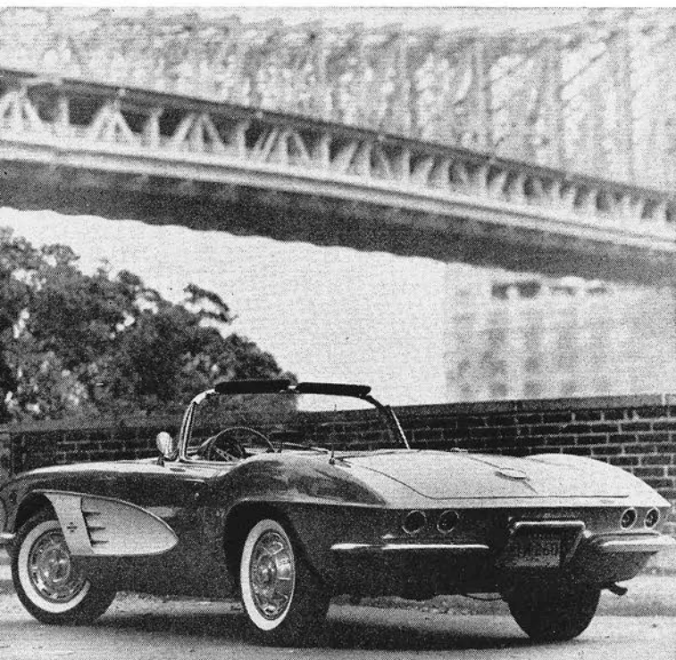
Upswept tail resembles XP-700, ties design to Corvair styling. Exhaust pipes end behind wheels, shouldn't get bent on steep driveways or curbs.
