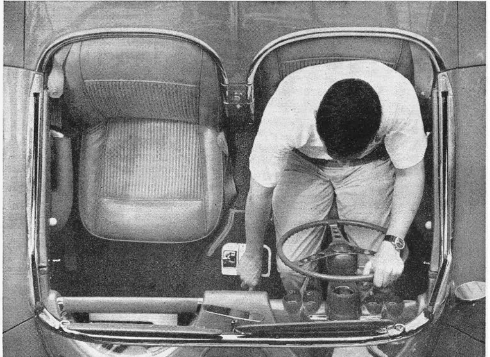
Cockpit continues emphasis on high style. Subtle changes over the years have brought more leg room, improvements in driving position. Seats look more buckety than they are, offering little side support.
