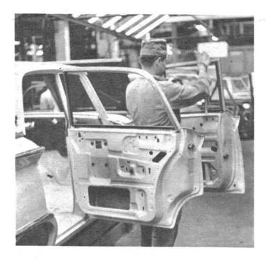
Still on the trim line, the body moves to the glass installation area. At the point shown here, the car is receiving the front door glass. Ford Motor Company makes a major portion of the plate glass used in its cars.
