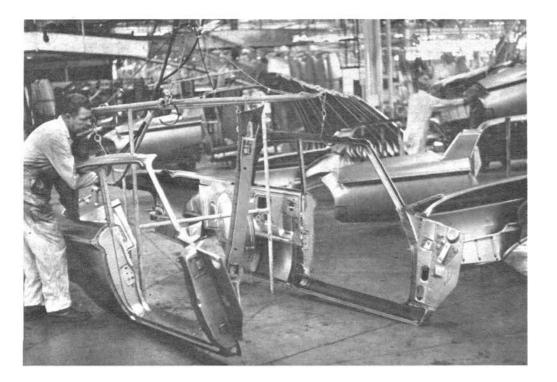
Two completed but separate side panels—right and left—have come off the conveyor. They will be placed on a hoist and taken to a jig, or body buck, to be welded to other parts to form the body shell.
