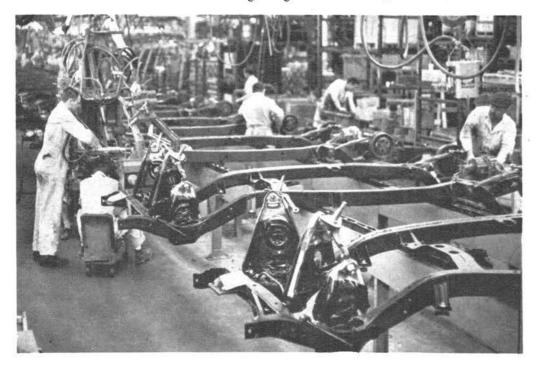
moved into position from the storage area and placed at intervals, upside down, on the moving conveyor.
