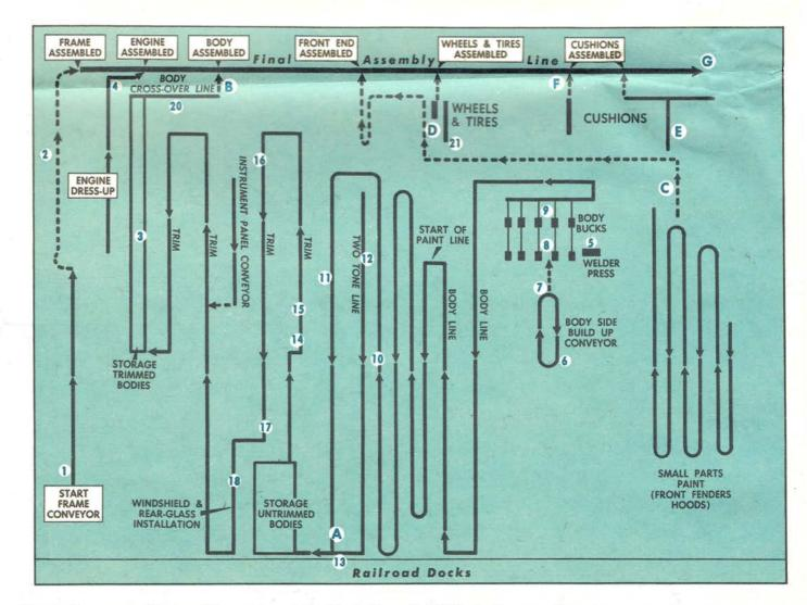
Here's the automobile-assembly section of the Ford plant. Solid black lines are floor conveyors; dotted black lines are the overhead conveyors. Numbers are operations shown in photos on following pages. Letters are color photos.
