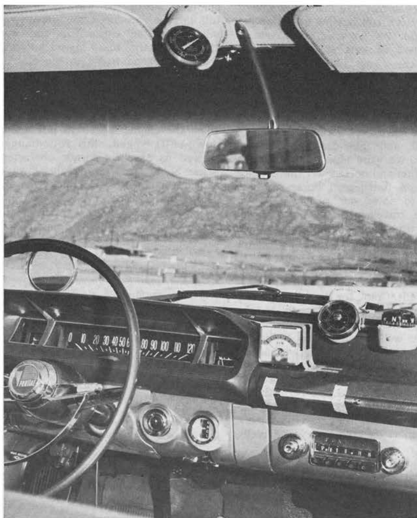
Instrumentation included Taylor outside thermometer on windwing (left), inside thermometer taped to cowl, combination altimeter and barometer, and compass. Other test aids were Dixon electric tachometer, Bowmonk G-meter dynameter.
