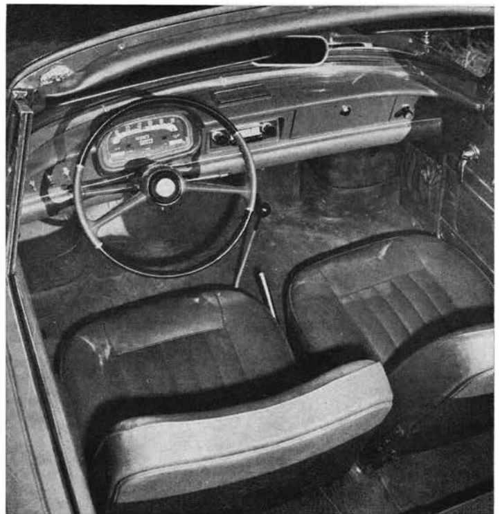
Due to the relocation of seating arrangements, the Caravelle allows better seat-to-wheel-and-gearshift relationship than the Dauphine.
