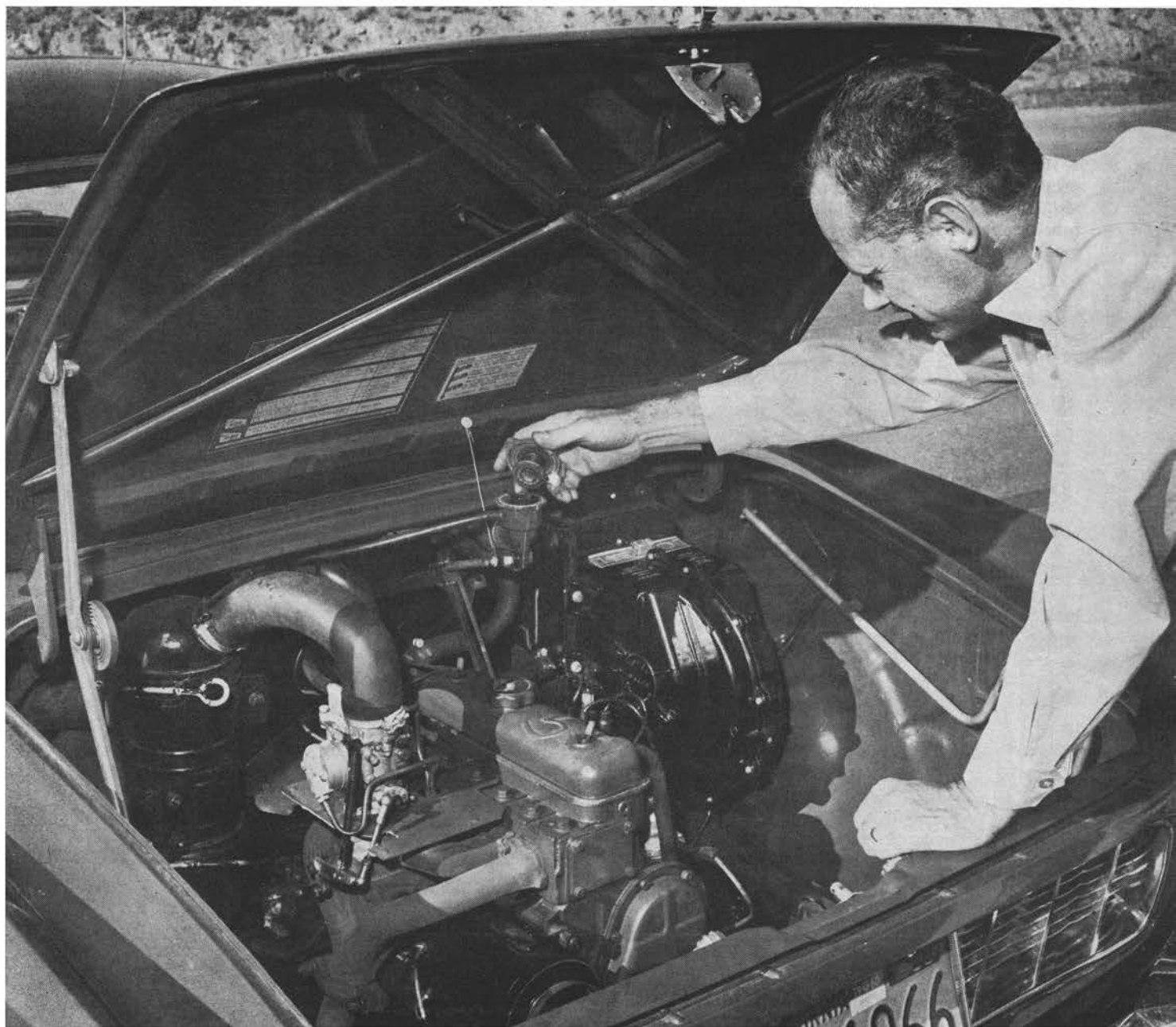
Although the Caravelle powerplant is essentially the same as that used in the Renault Dauphine, some additional horsepower has been gained through compression and carburetion change. In the 798 miles of maximum-effort driving, we averaged 31.1 mpg.
