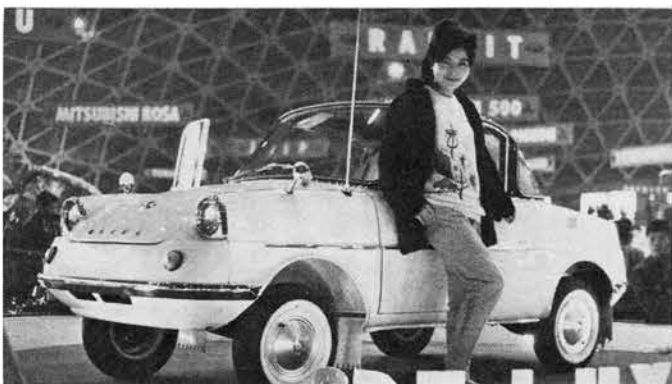
Rear-engined Subaru features unitized construction, independent suspension, and a very small 16-hp, 356cc, vertical-twin mill.
