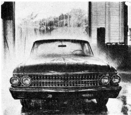
Ultra high-pressure wash at Ford Engineering showed test Galaxie was free from leaks, well-built.
