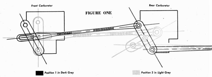
to the front carburetor has been altered by grinding a notch (b) ½ inch from the back of the slot. The lever (c) and the control cable (d) both ride the carriage, as shown. The spring (e) is attached to the end of the lever (f) and to the carburetor spring clip on the engine. When you pull out the knob with the engine at idling speed, check that the hook on the lever reaches the notch in the linkage rod. Mount the knob of the control cable under
