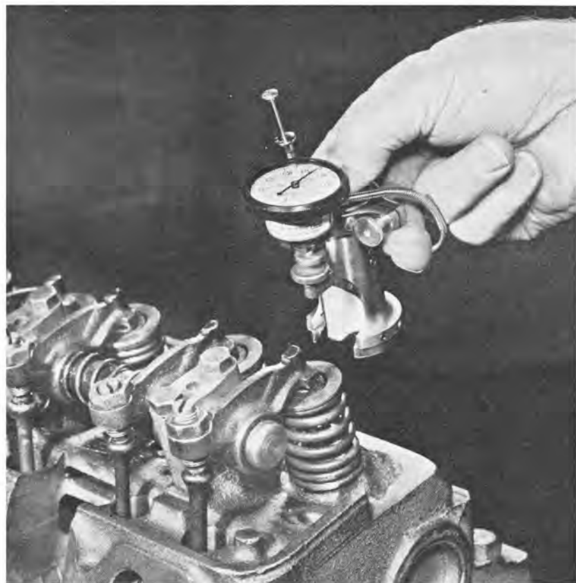
Part of the secret of the Valve Gapper's accuracy is the dial indicator. The outer case fits against valve spring retainer, spring loaded inner barrels fits under end of rocker. When maximum clearance is reached, a push on the attached cable brake locks indicator needle for an easy reference.
