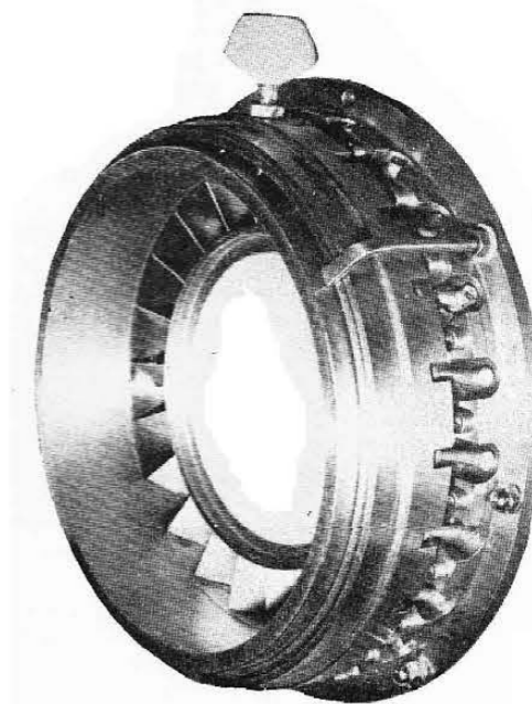
Assembly above is early variable-nozzle ring, placed between compressor and power turbines and marked by key 5 below. On this display unit the vanes or "nozzles" are actuated by turning the control ring — and thus the vane levers — by moving the white knob at the top.
