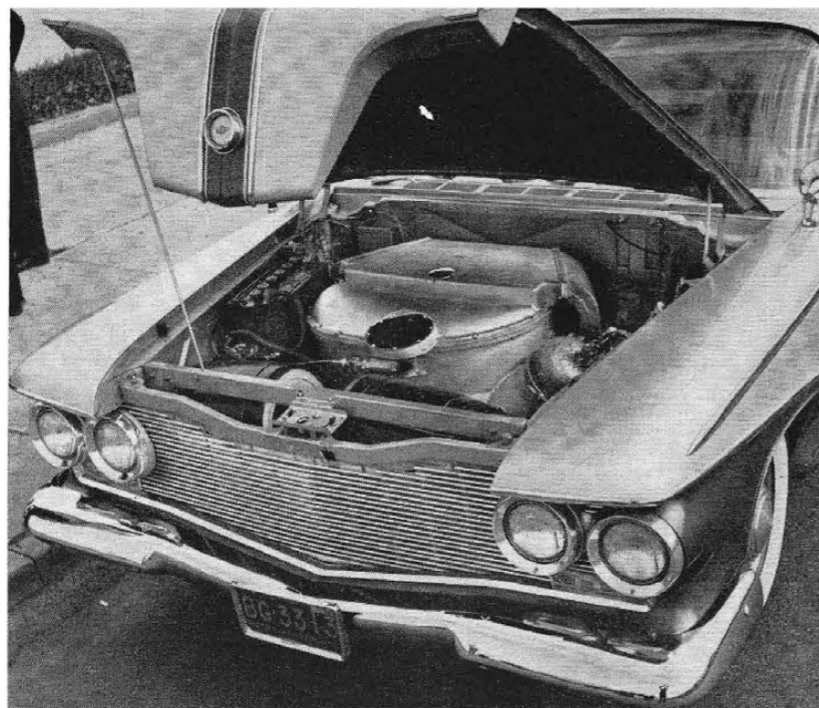
Steam car enthusiasts, take heart! With its welded steel case, the new turbine has a boiler-room look. Two big cylindrical air cleaners sit horizontally just behind the mildly restyled grille.
